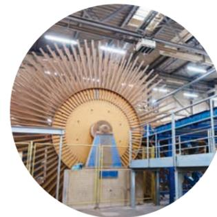
**3** The dried fibres are spread into a fibre mat and pressed in a hot press with a thickness of between 1.5 mm and 22.0 mm. The finalised continuous fibreboard is then cut to the desired lengths and cooled.
